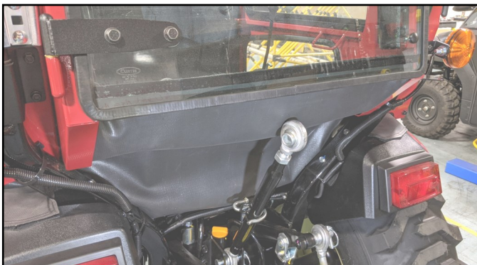
Fig. 21.6b (Secure Filler to Rear Panel)
