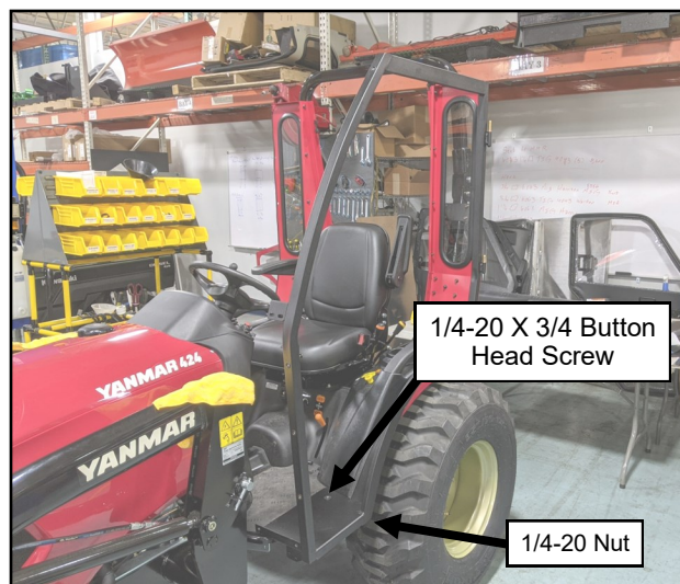
Fig. 4.2 (Install Left Side Frame)
