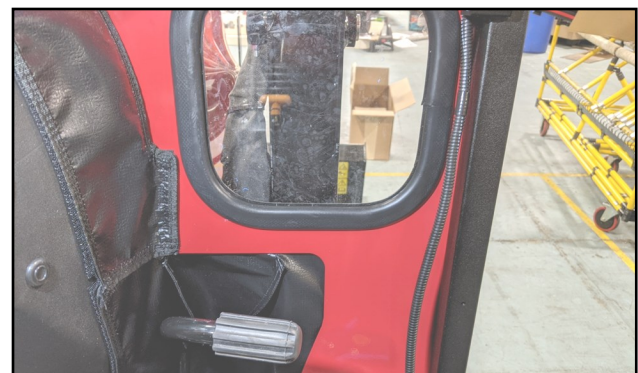
Fig. 15.5 (Harness Runs Down Side Frame)
