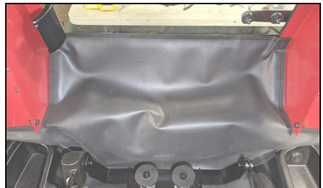
Fig. 21.6a (Secure Filler to Rear Panel)
