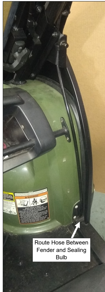
Fig. 7.1b Drain Hose Routing
