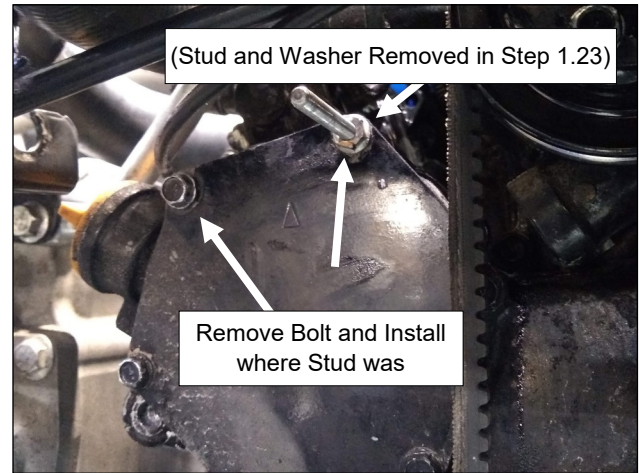
Fig. 1.25 Engine Cover Fasteners
