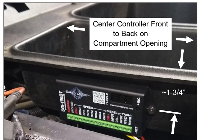
Fig. 5.3 Controller Mounting
