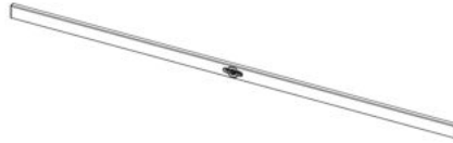
CROSS TUBE ASS'Y. (REF.: 68" LG.) P/N: 8SV-113-00234 (QTY.: ONE)
