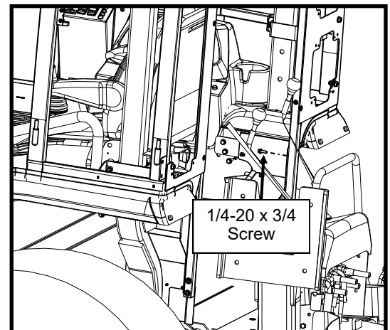
Figure 7.3b: Right Rear Corner Filler
