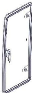
SIDE WINDOW ASSEMBLY, RIGHT P/N: 8SV-K6247-12R
