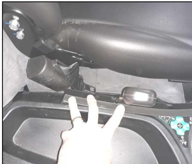
Figure 3.1a (Mark Brush Mounting Holes)
