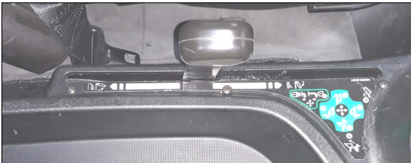
Figure 3.5 (Install 3-Point Hitch Lever Brush)
