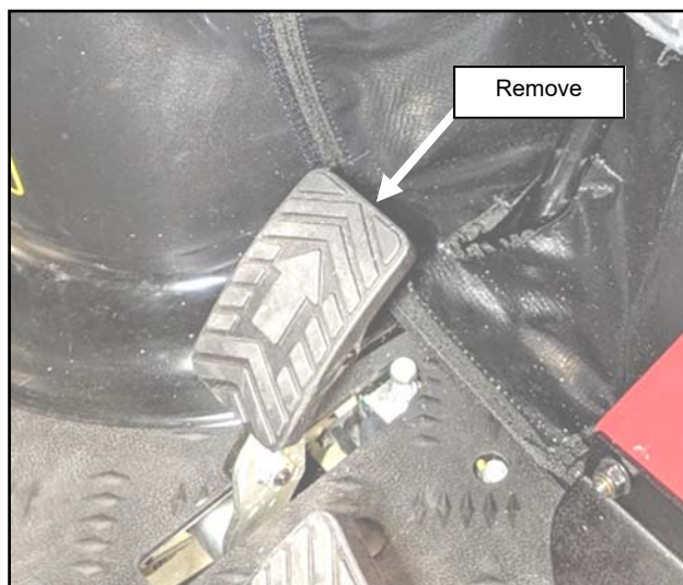
Figure 2.1 (Remove Forward Pedal)
