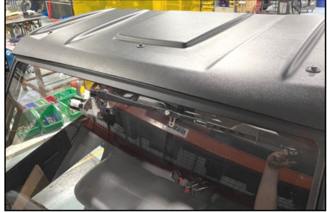
Fig. 2.3 (Install front screws, washers & lock nuts)
