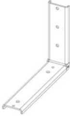
TOOLBOX SUPPORT BRACKET, LARGE P/N: 8SV-WA-00363 (QTY.: 2)
