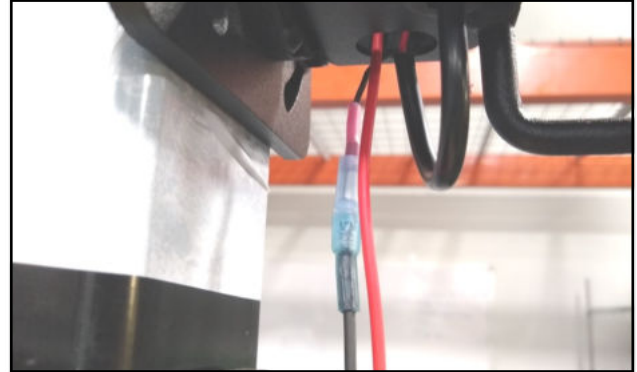
Fig. 10 (Black Wire to Light Connection)
