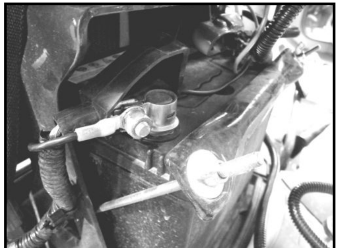
Figure 16: Install Black Wire
