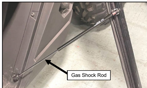
Fig. 1.6 (Install Gas Shock on Door)
