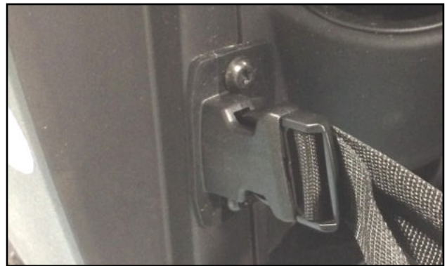
Fig. 1.2 (Remove Left Net-Clip)
