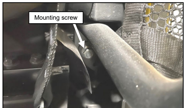
Fig. 1.4 (Remove Left Net Mounting Screw)
