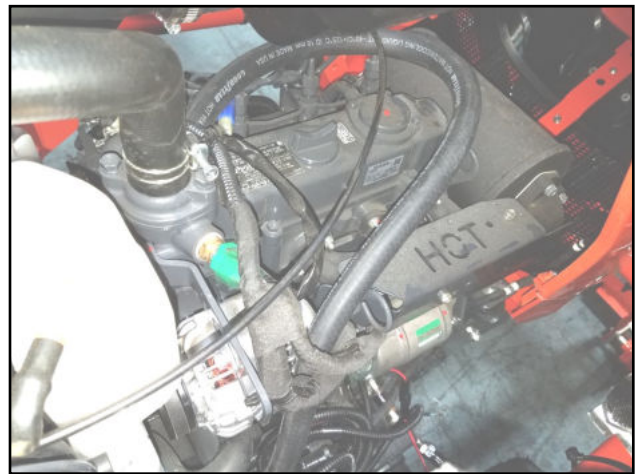
Figure 2.8 (Run Hose Around Engine) (View from Right Side)
