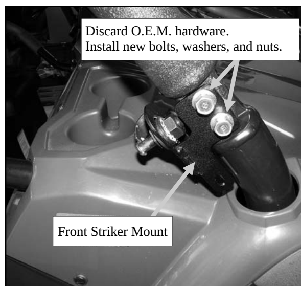
Fig. 3.1 (View of front right corner)
