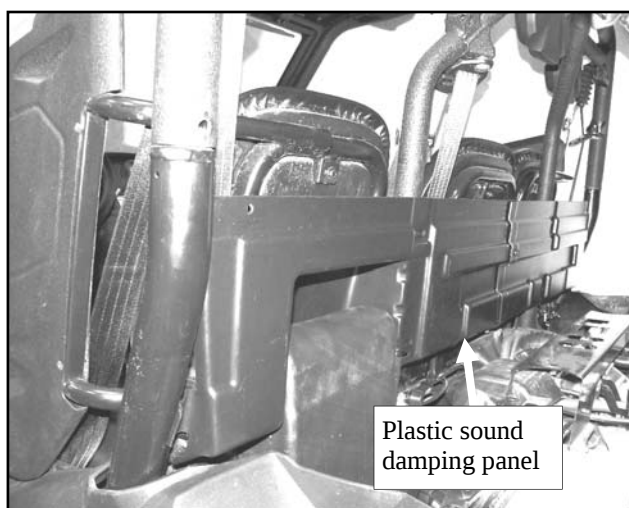
Fig. 1.3 (Rear plastic sound damping panel reinstalled)
