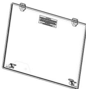
RADIATOR SHROUD ASSEMBLY P/N: 8SV-111-00032
