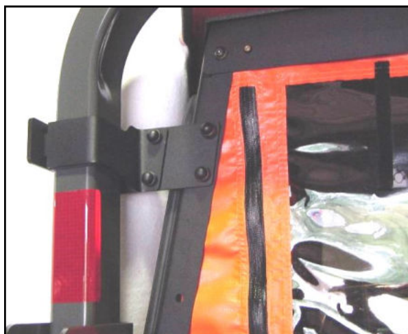
Fig. 6.2 (view of left side of tractor) ( upper roll bar mount shown here)
