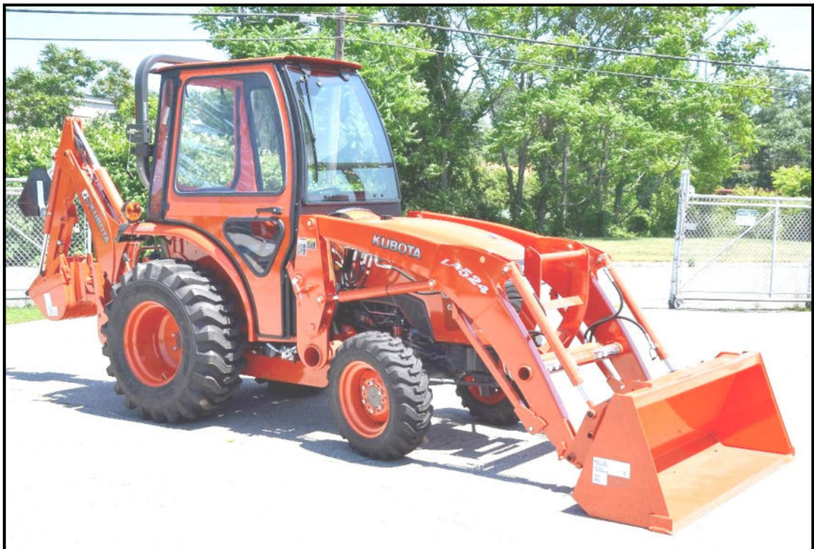
Hard sided cab shown here. Available options are: heater, work lights, and rear window wiper. Note: a front windshield wiper comes standard with this cab kit.
