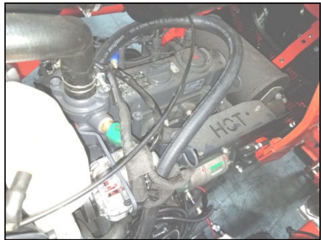
Figure 20.8 (Run Hose Around Engine) (View from Right Side)
