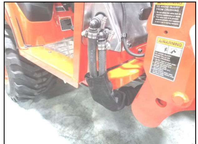
Figure 20.10 (Connect Hoses to 90° Elbows)
