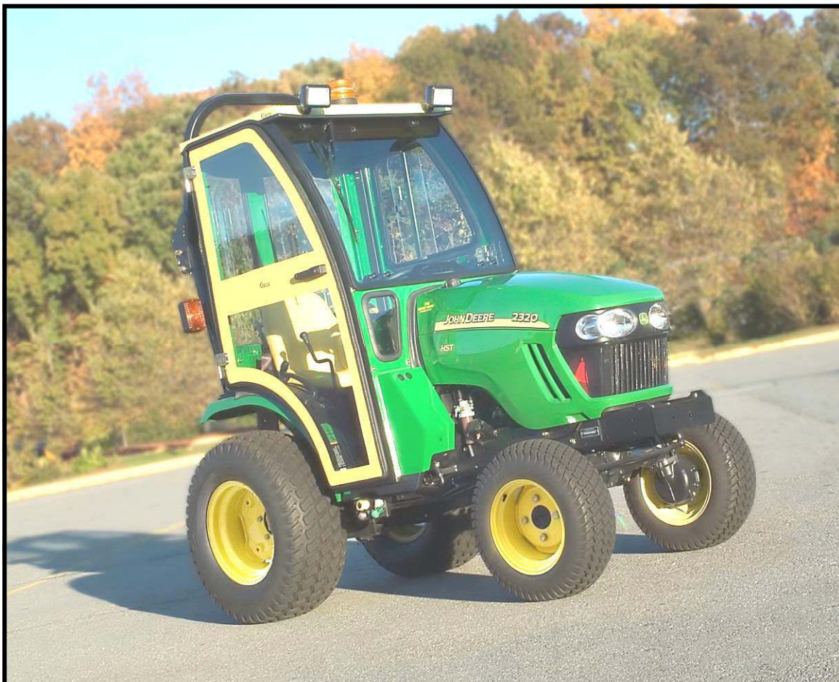
Note: soft sided cab shown on model 2320 with optional work lights and optional strobe light.
