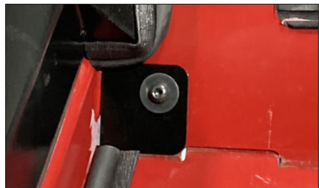
Fig. 10.6 (Left floorboard filler panel)
