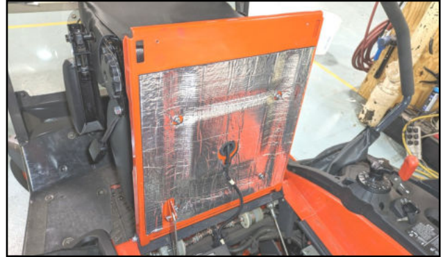
Fig. 10.4 (Under Seat Insulating Panel)
