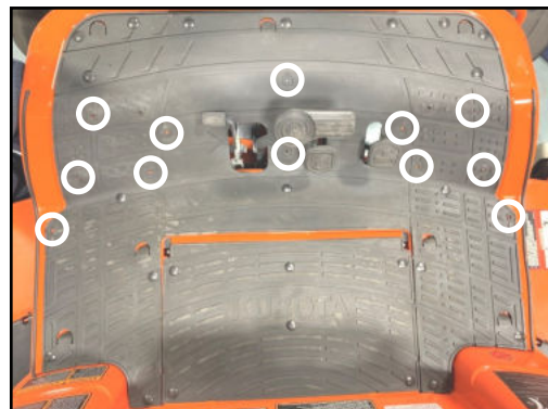
Fig. 4.3 (Remove Pine Tree Clips)
