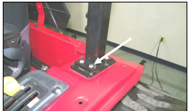
Fig. 1.11 (Replace ROPS Screw)
