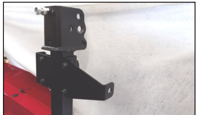
Fig. 3.1 (Attach ROPS Clamp Brackets)
