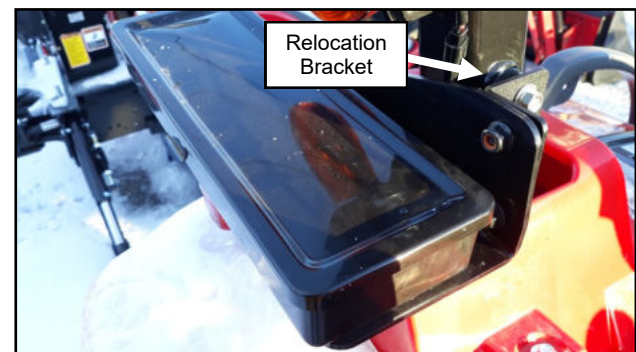
Fig. 26.4 (Install ROPS Mounted Toolbox)
