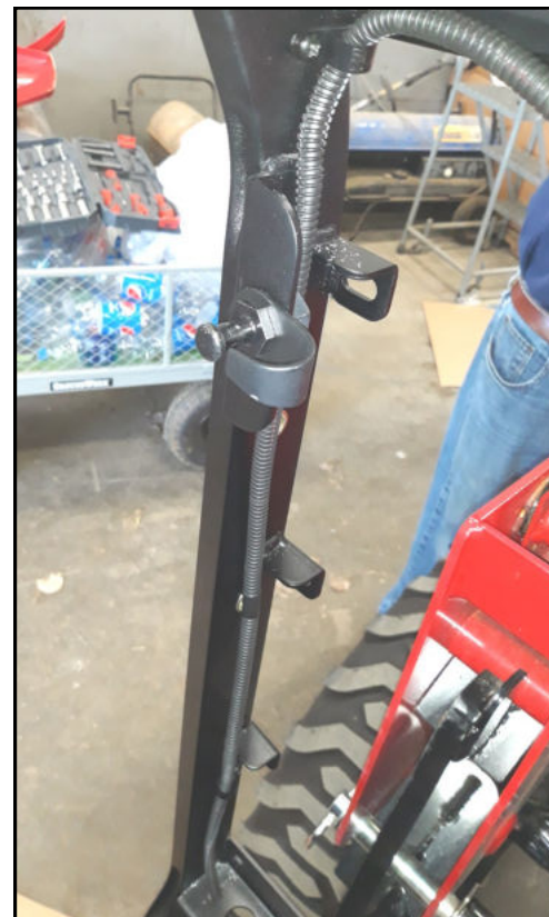
Fig. 8.4 (Run Wire Harness Down Side Frame)
