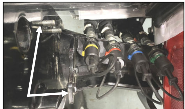
Fig. 1.13 (Unbolt Hydraulic Bracket)
